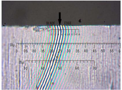
The T10 microscope is supplied complete for T10 blade thickness measurement with:
