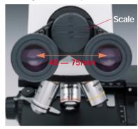
adjustment and diopter setting. High eyepoint design eyepieces with F.N.18 can be used comfortably without removing eyeglasses.
