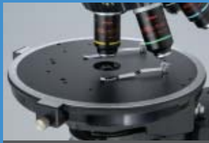
High-precision rotating stage (LV100POL)
