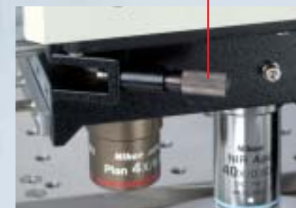
Parfocal distance correction knob
