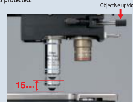
Objective retraction mechanism
