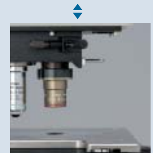
Front/back sliding objective changeover
