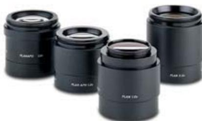
The 2× planapochromatic objective can produce a total magnification of 500× when used with 40× eyepieces. It has a numerical aperture of 0.2 and a resolution of 615 line pairs per millimeter. The working distance of the 0.5× plano objective is 135 mm, offering ample space for tools to manipulate the object. All objectives are lead-free.
