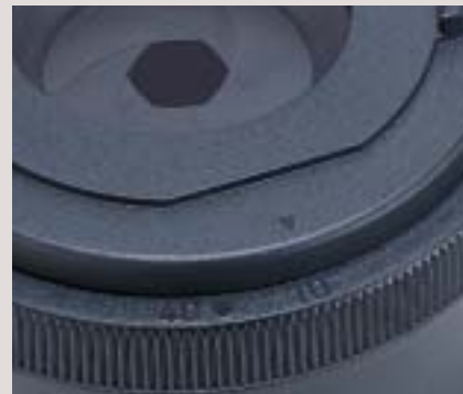
Field diaphragm with position-guide markings.
