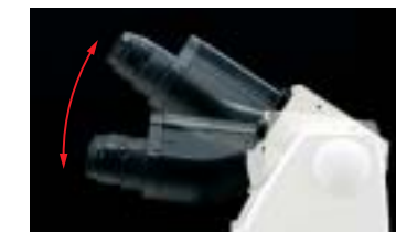
Tilt angle is adjustable 8°–32°.
