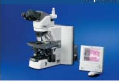
ECLIPSE 80i configured with ergonomic tube, DSC port, and digital camera DS-5M-L1.
