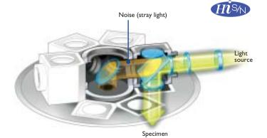
Stray light is thoroughly eliminated from the optical path in the filter turret.
