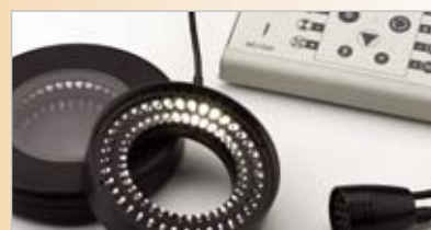
Laser emitting diode, illuminations, transmitted-light base, ring illuminator and spot
