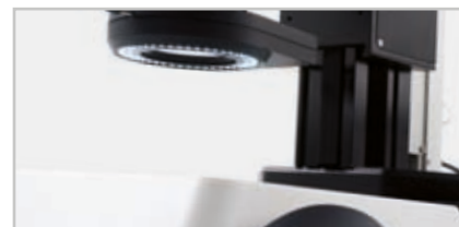
Planapo 1x: the working distance of 61.5mm leaves a lot of free space under the objective
