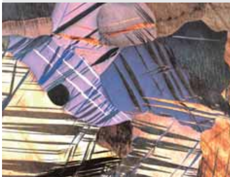
Cast tin with deformation twins, 200 x
