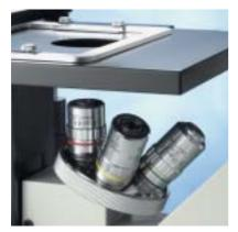
Nosepiece inverted microscope
